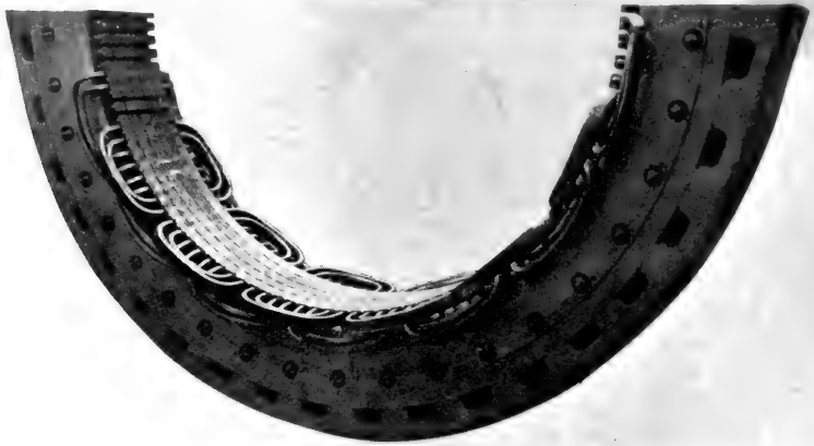
FIG. 248.—Dick, Kerr & Co. Alternator. Three-phase, Half-coiled, Double-coil, Two-slot Spiral Winding in two ranges.
